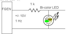
Set the frequency to 1 Hz and amplitude 10 V. Use Sine, Triangle and Square wave sources. What frequencies cause the LED to appear "on" continuously?
