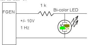
Set the frequency to 1 Hz and amplitude 10 V.
