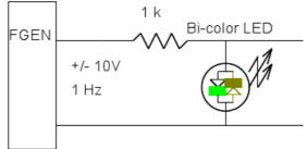
Set the frequency to 1 Hz and amplitude 10 V.
