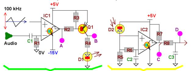
PWM Modulator + IR Emitter IR Detector + PWM Demodulator
